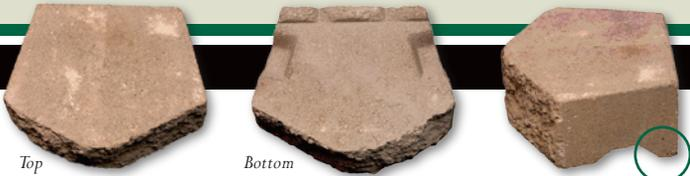
NurseryStone's bottom heel enables the block to hook over the course below, securing the block and providing the proper set-back for a solid, professional finish.
