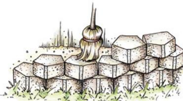
**STEP 4:** Continue leveling from side-to-side and front-to-back, compact loose dirt behind the wall.
