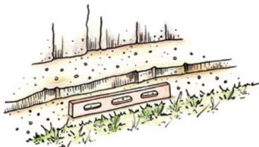
**STEP 1:** Begin at the lowest elevation. Determine line and height of wall. Dig a trench 4" deep and 12" wide. Fill the trench halfway with level, compacted gravel.
