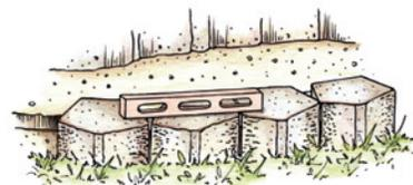
**STEP 2:** Install first course of blocks. Check for level side-to-side and front-to-back. Fill between and behind the blocks with gravel. Brush excess gravel from top of blocks.
